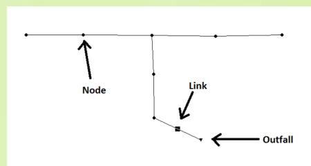
Fig. 3: Nodes, links, and Outfalls in the SWMM model
