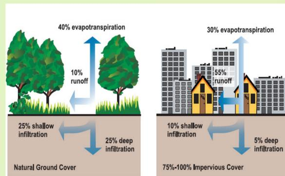
Fig. 1: Effect of impervious cover on runoff and infiltration rates in urban areas.
