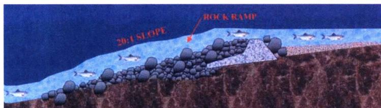
*A rock ramp, showing how fish can swim over a dam without removing it.*
