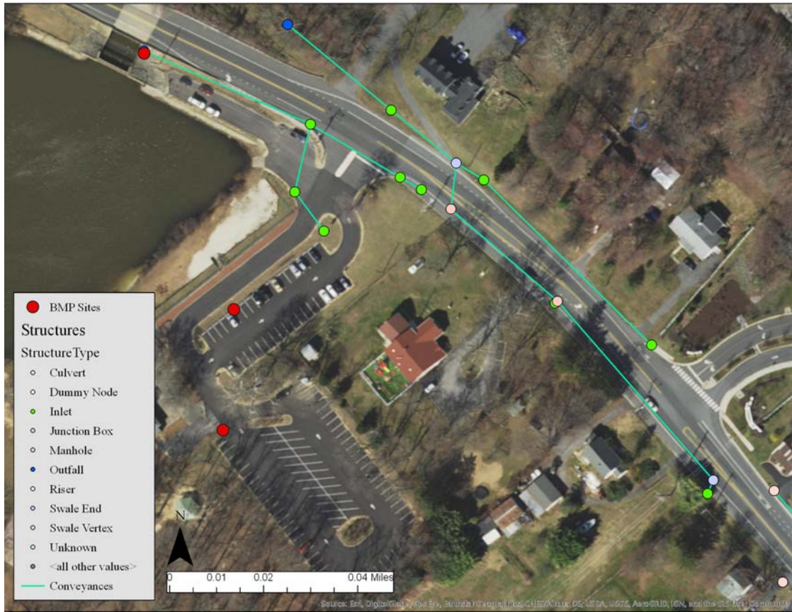
Figure 3.5: Stormwater conveyances with the best management practice sites
