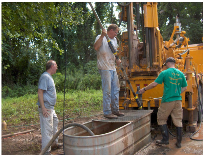
Dr. McLaughlin and co-workers set up the sonic tool to run the geophysical log at the Summit Marina site. (Photo by DGS staff)
