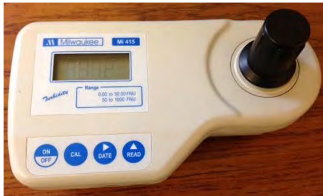
Figure 3.4. Turbidity meter, University of Delaware
