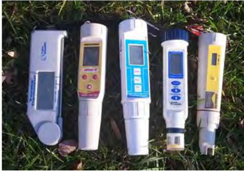
Figure 3.1. Water quality probes (Left to right: temperature, pH, DO, and conductivity from Wilmington; TDScan conductivity from University of Delaware) Monitoring probes from the City of Wilmington (pH, DO, temperature, conductivity) and University of Delaware (TDScan 3 conductivity probe, turbidity meter) - Figures 3.1 and 3.4
