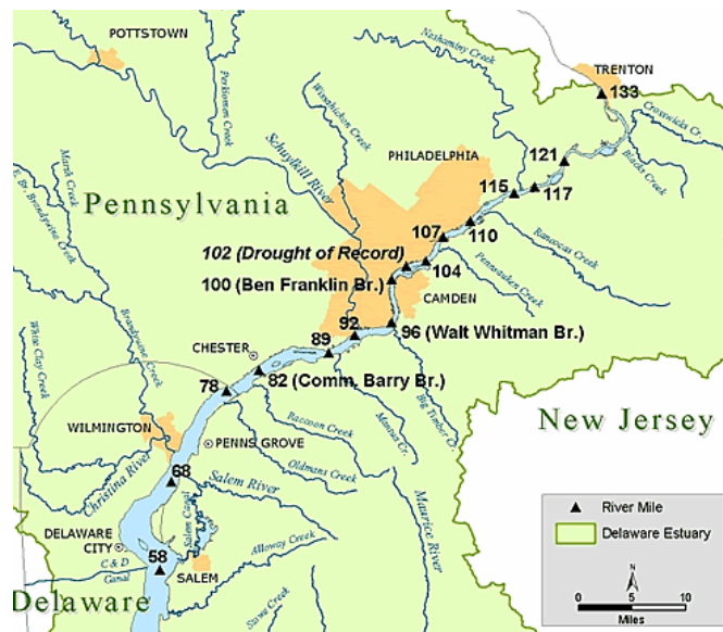
Figure 6.36. Salt line location along Delaware River during the 1960s drought of record.
