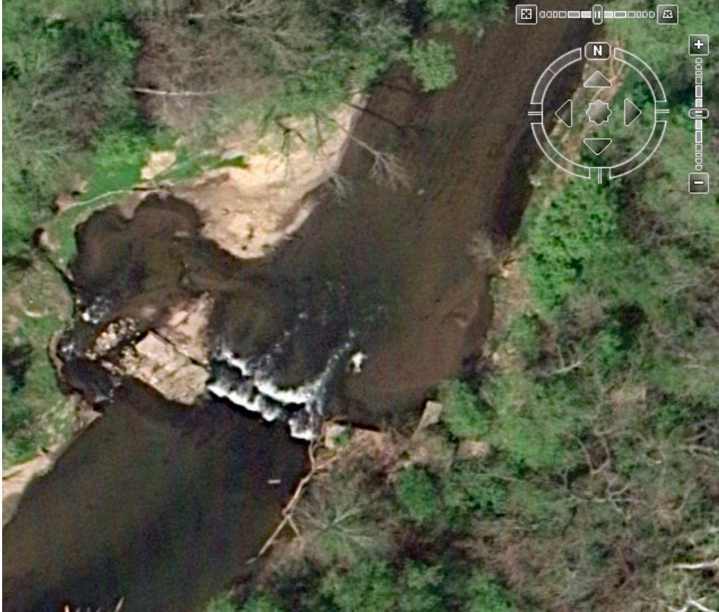
Photo 3. Plan view of White Clay Creek Dam No. 1. Note breach along overbank to left.
