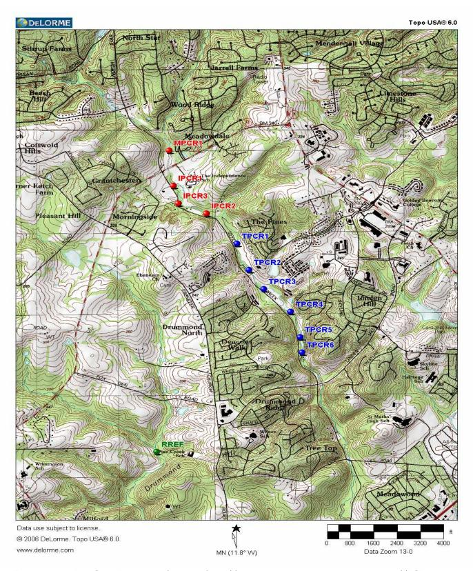
Figure 10. 2006 Pike Creek Restoration Sampling Sites. The 5000 linear feet restored segment sites (TPCR 1-6) are indicated in blue. The 3200 and 400 linear feet unrestored reach sites (IPCR 1-3 and MPCR 1) are indicated in red. The 2006 regional reference (RREF) is indicated in green.
