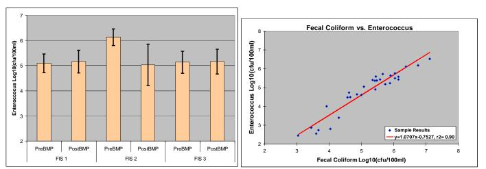
Figure A1-3. Storm-flow Enteroccocus concentration and the relationship between log transformed Enteroccocus concentration and Fecal Coliform concentration at all Fisher Farm sites and sampling dates. Post BMP mean Enteroccocus concentration is less than pre BMP mean Enteroccocus concentration (p<0.05, one tailed test).
