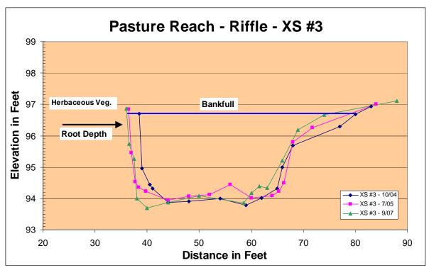
Figure A1-5. Riffle Cross-section in pasture reach.
