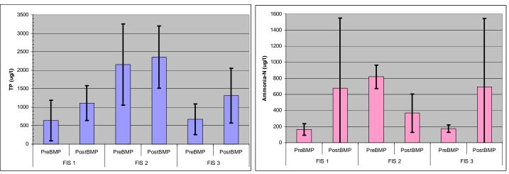
Figure A1 -1. Storm-flow Total Phosphorous and Ammonia concentration at FIS1,FIS2, and FIS3. Post BMP mean ammonia concentration is less than pre BMP mean ammonia concentration at FIS2 (p<0.05, one tailed test).
