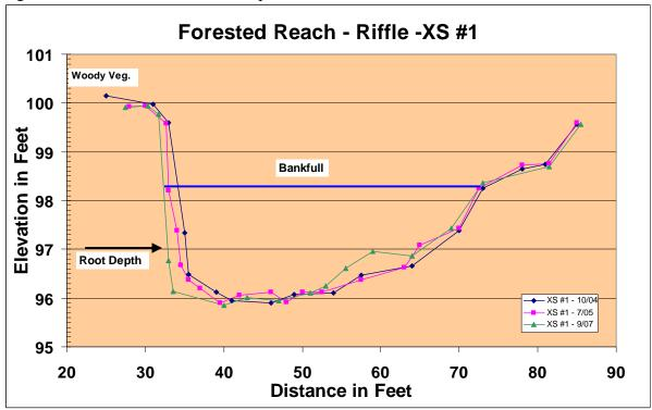
Figure A1-6. Riffle Cross-section in forested reach.
