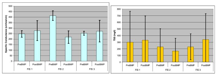
Figure A1-2.. Storm-flow Specific Conductance and Total Suspended Solids at FIS1,FIS2, and FIS3. Post BMP mean Specific Conductance is less than pre BMP mean Specific Conductance at FIS2 (p<0.05, one tailed test).
