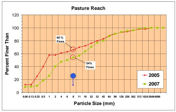
Figure 4 Stream bed particle size distribution in the forested reach prior to (2005) and following (2007) BMP installation.
