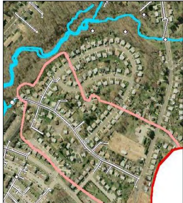
Figure 6: Outfall retrofit sites can be discovered by overlaying storm drains, streams and adjacent open land.
