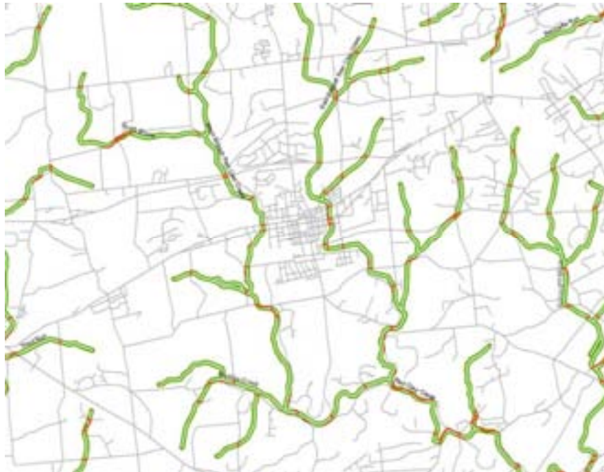
Figure 5.19. Road density within stream buffers in the Delaware River Basin.
