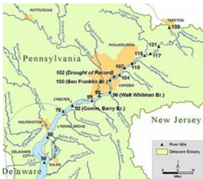
Figure 6.45. Salt line location along Delaware River during the 1960s drought of record.
