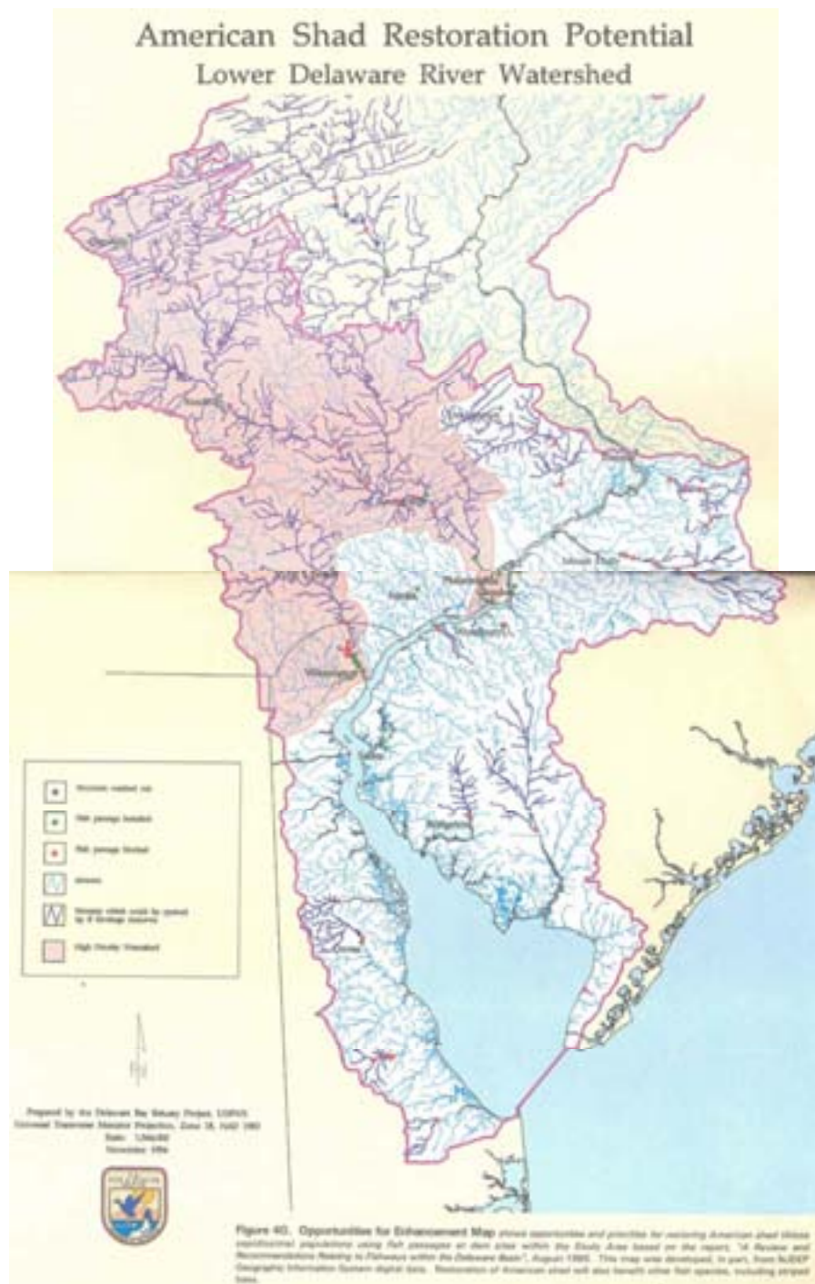
Figure 7.27. American shad restoration potential based on dam removal in the Delaware Basin (Partnership for the Delaware Estuary and USFWS 1996)
