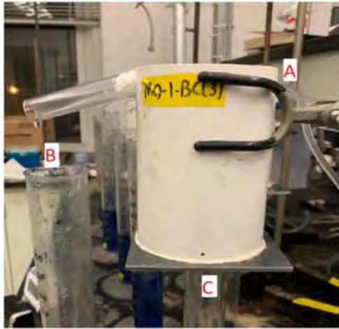
Figure 2: Infiltration test setup.
