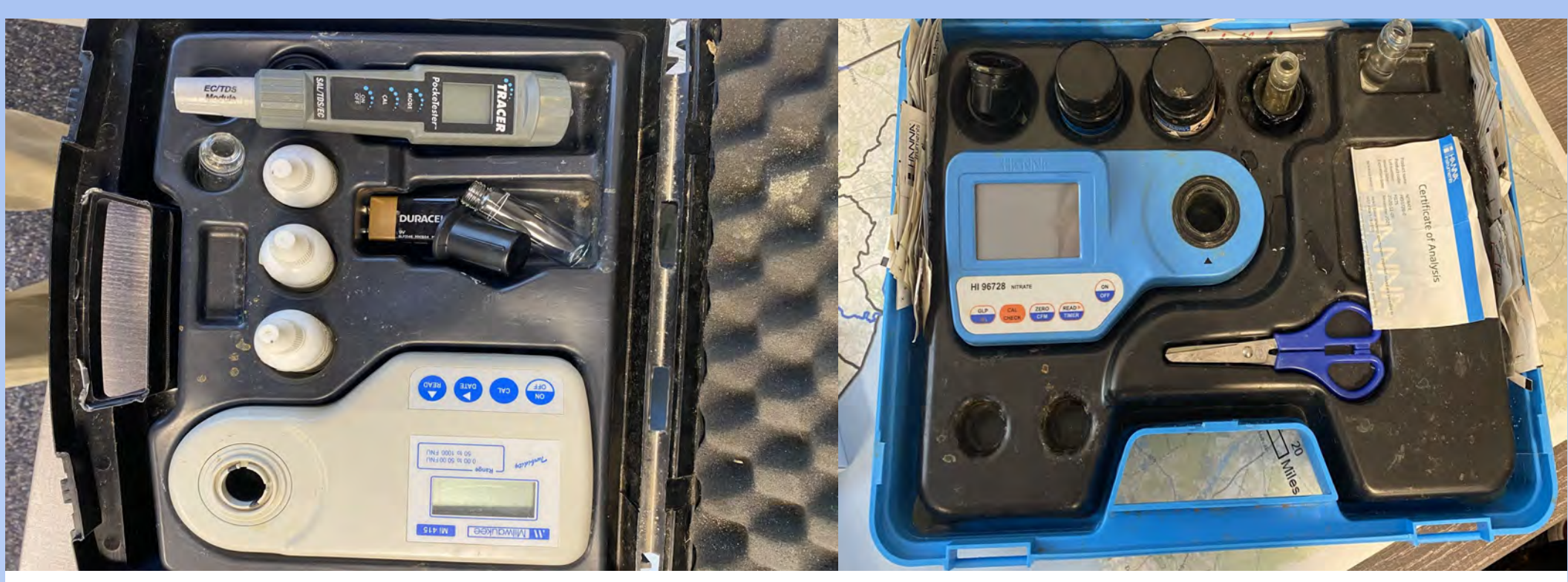
Fig. 1 Water Quality monitoring equipment; Nitrogen and Turbidity meters
