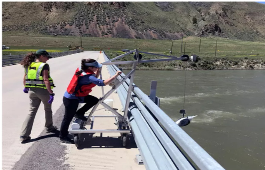
Figure 4: Researchers sample the Yellowstone River using a suspension sampler with a one-liter collection bottle
