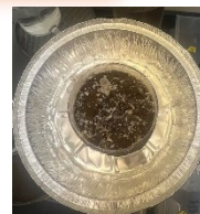
Figure 2. Photo of efflorescence from Mariotte bottle system
