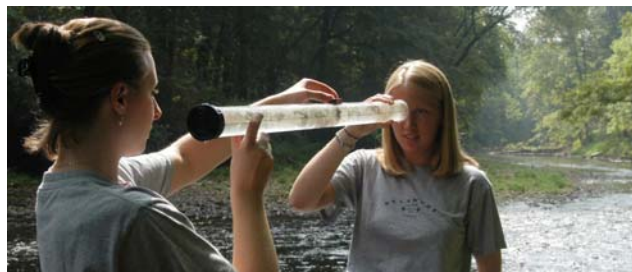
Ms. Cormier and Ms. Sentoff measure turbidity in White Clay Creek
